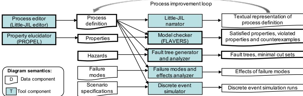
Fig. 1. A framework for iterative process improvement
