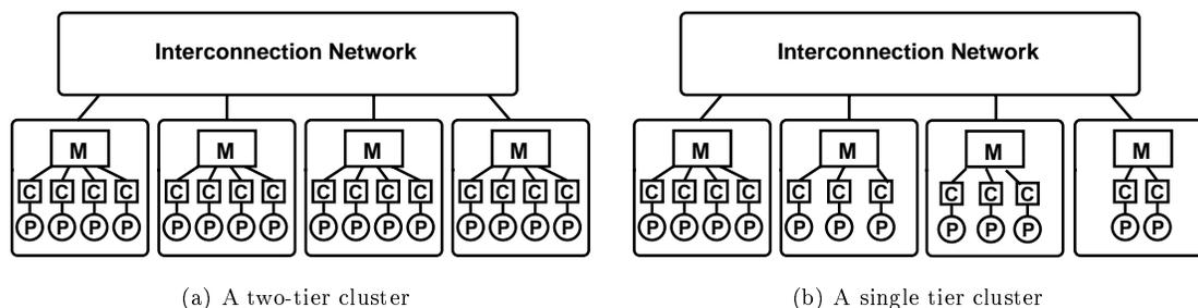
Figure 1: Block diagrams of a homogeneous (a) and homogeneous (b) dual tier clusters. M=memory, C=cache, P=processor. On-processor cache memories are not shown.
