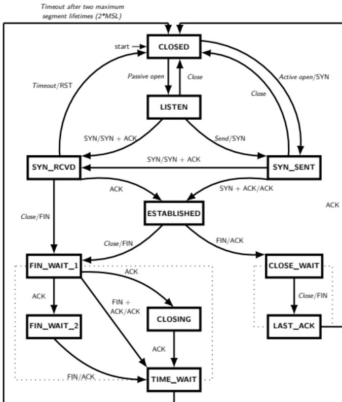
Figure 2: TCP State Diagram
