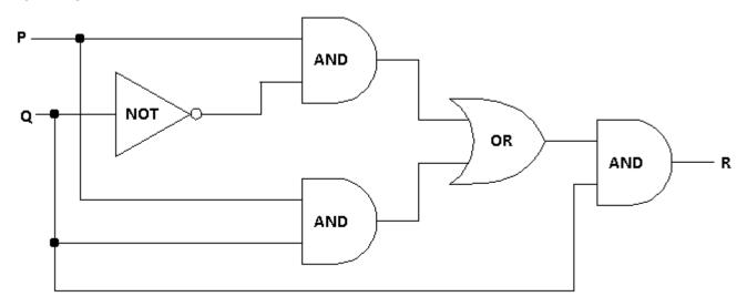
8.1. Simplify the above digital logic circuit using propositional algebra.
