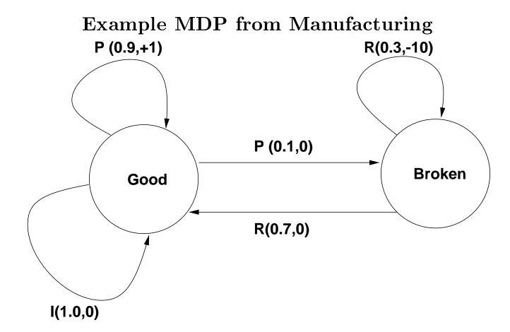
Machine can be in a good state or broken. Producing a part gives a reward, but ages the machine. If the machine fails, it costs some money to fix it.
