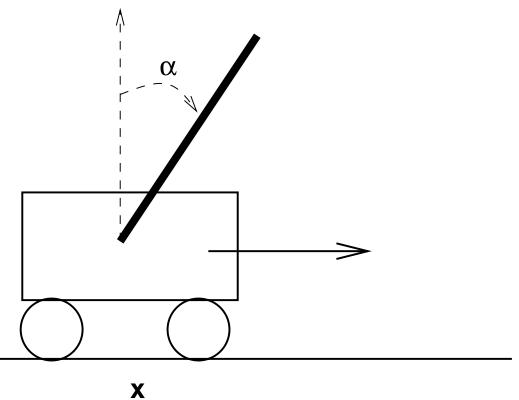
Goal is to keep pole balanced for as long as possible. States are position of cart, angle of pole, and velocity and angular velocity of cart and pole. Actions are apply force to the left, and to the right.
